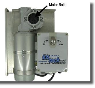
7. Install Motor Bolt and Washer. Tighten Motor Bolt to Approximately 70 Foot Pounds.
