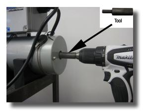
In Case of a Power Outage. This Tool May be Inserted Into a Drill to Raise or Lower Your Lift. First Remove Rubber Cap From Motor Shaft.
