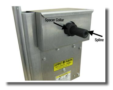
5.Install Spacer Collar and Spline.
