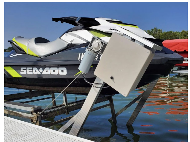
Example of finished installation on cantilever lift
