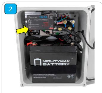
Secure the solar charge regulator anywhere inside the box
