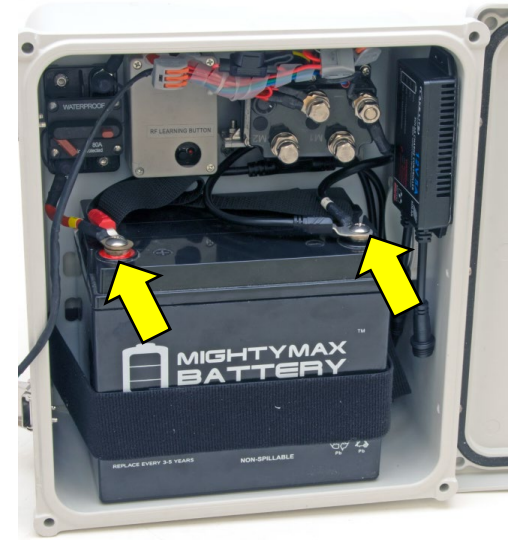
Connect the power cables for both motor & solar charge regulator to the battery terminals
