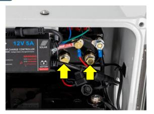
Connect the motor wires to the contactor study labeled M1 & M2:
