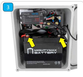
Connect the power cables for both motor & solar charge regulator to the battery terminals
