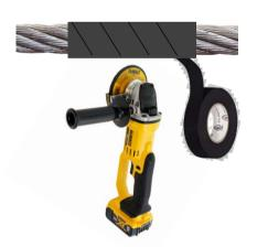
Wrap the cable cutting area with tape to ensure a clean cut.
