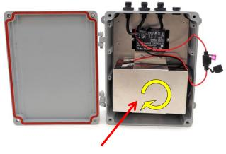
The battery should be mounted in the most upright position. If you mount the control box upside down remove the battery and flip it around so the battery will be up right after installing the control box.
