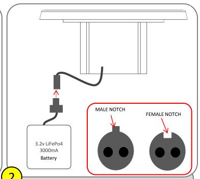
Connect Battery: Caution! When plugging battery connectors together, align notches before joining both connectors.
