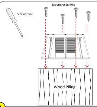
Place light onto piling and mark holes. Drill small pilot holes in piling with drill bit. Use screwdriver to secure the light to your piling with mounting screws – *Not Included*
