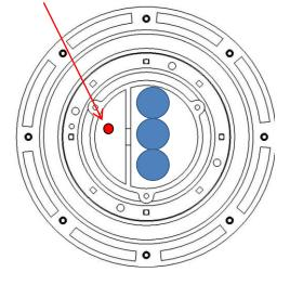
Look inside the light to see a small push button in order to select power level or on/off position.
