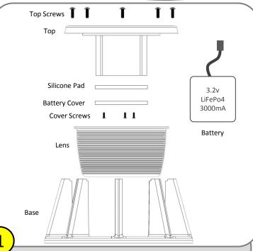
Use the provided wrench to separate your light: The battery is not connected when shipped.
