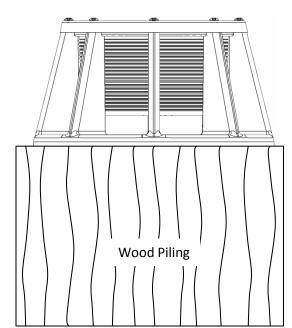
Verify that the top screws are tight to provide a good seal for the lens. Verify that the base of the light is secured to the piling.
