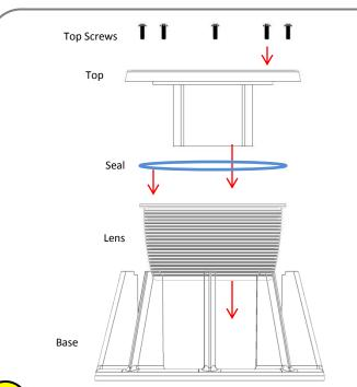
Use Provided wrench and top screws to assembly your light together. NOTE: The seal must be in the correct position before tightening down the top to the base.
