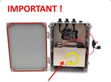
The battery should be mounted in the most upright position. 4 screws will need to be removed to allow the battery to be mounted inside the control box. If you mount the control box upside down remove the battery and flip, it around so the battery will be up right after installing the control box.
