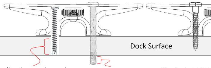
When using screws make sure you have enough length going into your dock surface to secure the cleat properly
