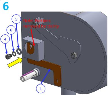
Place the curved hold-arm bracket behind the protruding box area and use the ¾" Bolt to secure in place. Note the larger slot will be mounted to the winchbox, the smaller slot will mounted to the motor.
