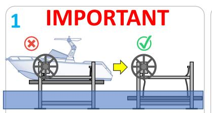
Fully lower the boat lift, remove the boat and any weight from the boat lift carriage. The cable should be slack. Ensure the lift carriage is fully down.
