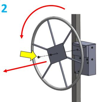
Remove the nut, washer, or bolt holding the wheel on. Turn the wheel counter-clockwise to unthread the wheel from the winch shaft. NOTE: if the wheel is rusted to the shaft try holding the shaft to prevent the shaft from turning while you turn the wheel to break free.
