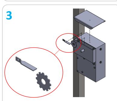
Remove the top cover and then remove the break dog and brake disc. These items will no longer be used. Reinstall the top cover when finished.
