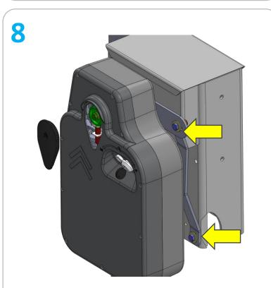
Make necessary adjustments to motor torque arm and hold arm positions then tighten all bolts & nuts securely.
