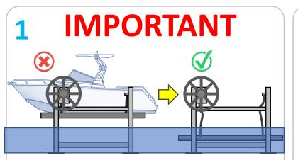
Fully lower the boat lift, remove the boat and any weight from the boat lift carriage. The cable should be slack. Ensure the lift carriage is fully down.
