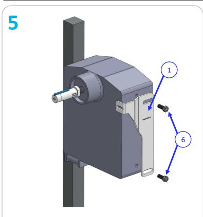
Attach the hold arm to the right corner of the winch box as shown. Leave fasteners loose.
