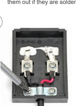
Replace the wire clamp with the hump facing downward
