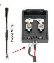
Insert diode wires, stagger the fork terminals for easy entry
