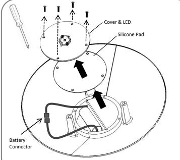
Use screwdriver to remove cover & silicone pad.
