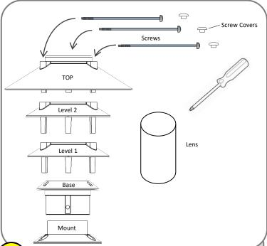
Use the long screws to assemble the light fixture.
