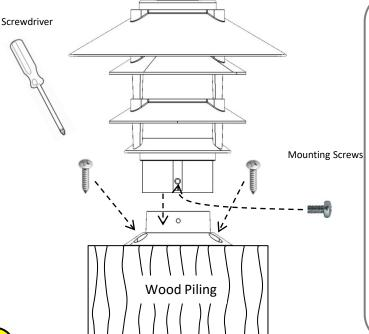
Place light onto piling and mark holes. Drill small pilot holes in piling with drill bit. Use screwdriver to secure the light to your piling with mounting screws – *Not Included*
