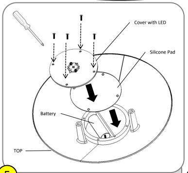
Use the provided screws to secure the silicone pad and cover. Fully tighten screws to ensure the chamber is water proof. Make sure wires are not obstructing the silicone pad.
