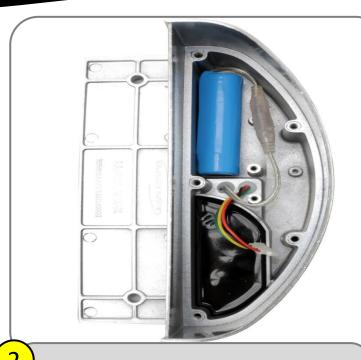
Connect battery with identical clear wire inside.
