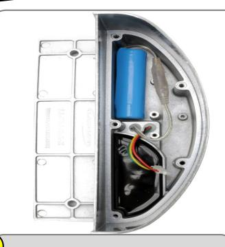
Connect battery with identical clear wire inside.
