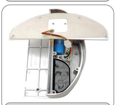
Connect the Light Cover: NOTE make sure to align the connector notches and red/black wire colors when plugging the two sides together.
