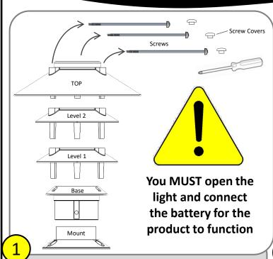
Use a screwdriver to separate your light fixture. The battery is **NOT** connected when shipped. You must connect battery for the product to function.
