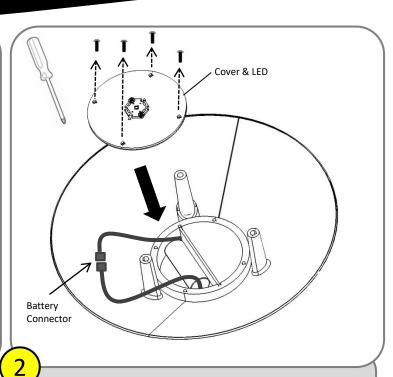
Use screwdriver to remove cover. Connect Battery & LED. Tuck wires neatly so they do not obstruct battery cover lip Reassemble battery cover and tighten securely.
